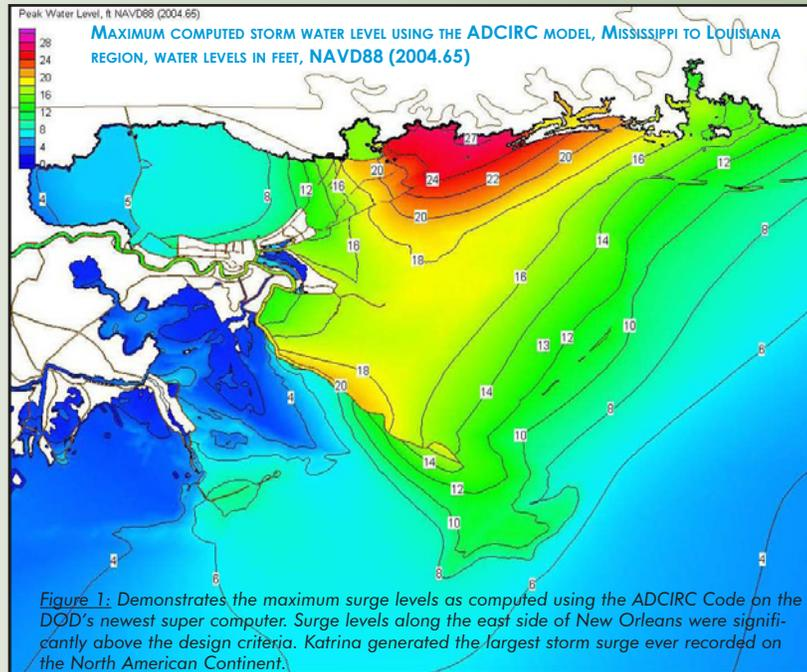
Figure 1: Demonstrates the maximum surge levels as computed using the ADCIRC Code on the DOD's newest super computer. Surge levels along the east side of New Orleans were significantly above the design criteria. Katrina generated the largest storm surge ever recorded on the North American Continent.
