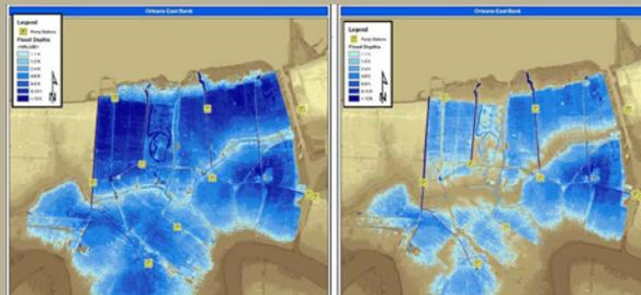
Figure 2: Demonstrates the reduced flooding that would occur if resilient levees and floodwalls were in place. For this section of Orleans Parish, approximately two thirds of the flood waters entered through breaches and one third from rainfall and overtopping. Resilient structures that would not breach when overtopped, would have reduced flooding by 2/3 and reduced losses by about one half.
